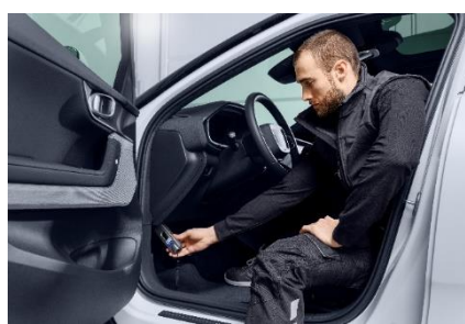
The final report integrates both data from the charging device as well as information from the OBD port.
